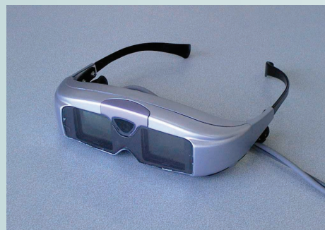
F Optical see-through HMD for outdoor use.
