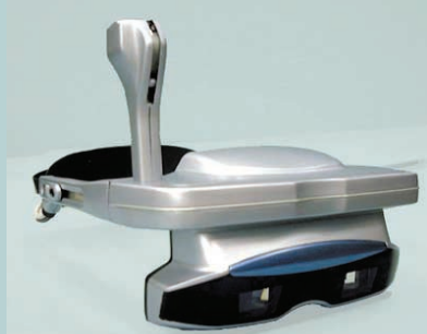
(2) COASTAR—parallax-free video ST-HMD. (1) Diagram of product. (2) Actual product.
