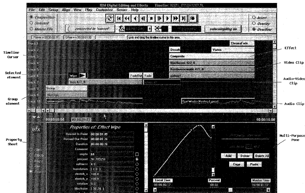
Figure 1. The primary EFX user interface. The timeline appears in the middle section. The interface is "malleable" in that (1) the multipurpose pane is reused for the Clip List, the Effects Palette, a text editor for modifying Effect Definition Files, a subwindow for server messages (errors and others), and the Property Sheet, and (2) the sizes of the timeline and the multipurpose pane are adjustable, ranging from the timeline being completely hidden to occupying the entire area they both now occupy.
