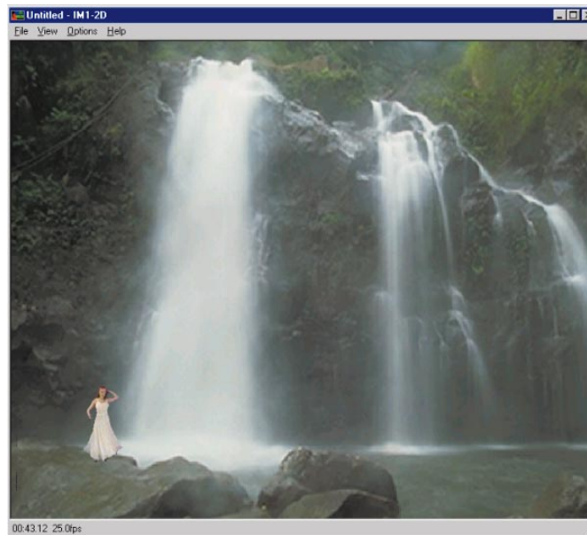
Figure 4. MPEG-4 Video showing a girl dancing in front of a waterfall. The background image is in JPEG format, while the girl is an MPEG-4 video object encoded from YUV and alpha raw stream.
