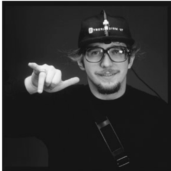
Fig. 5. A nearly-invisible head mounted display (HMD) and a hat-mounted camera to observe the user's hand gestures.
