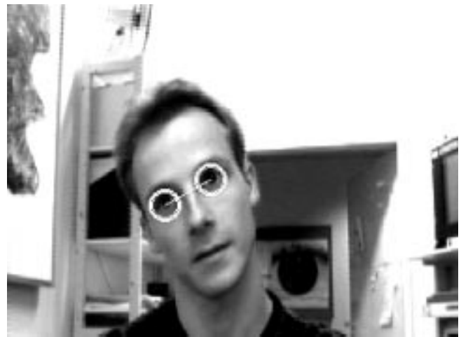
Fig. 14. Eyes are detected and tracked in a sequence of video images.
