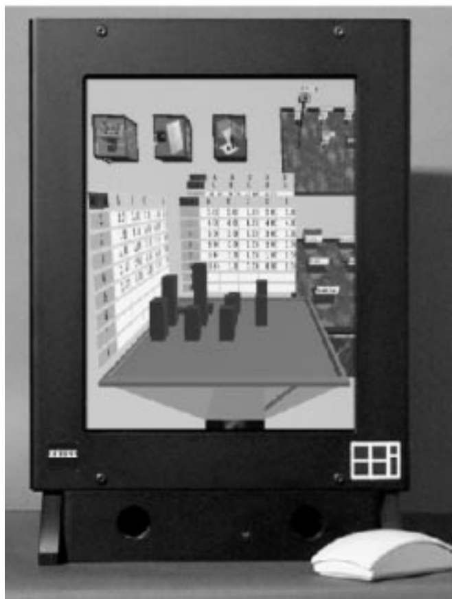
Fig. 8. Lenticular screen allows the separation of viewed 3-D images created in a raster-scan mode. The photo shows a 14-in XGA resolution prototype 3-D display developed for desktop applications.
